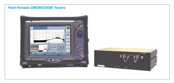
The CMA5000 OSA's are field portable DWDM/CWDM testers covering the 1250-1650 nm spectral range. Two OSA modules are available to meet all test requirements: OSA 400 and OSA 425.
